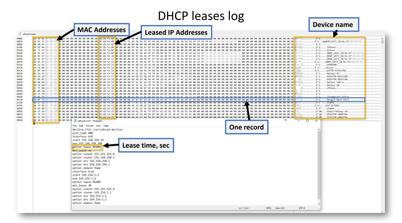
IP address rent-time is 24 hours, so all devices mentioned in the UDHCPD.leases file were connected to the network within 24 hours, starting from file creation date
