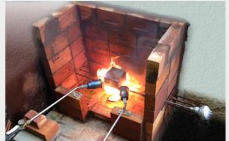
Sentinel Under High temperature fire test
