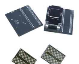
This adapter consists of one socket and two boards designed for BGA316 and BGA272 chips
